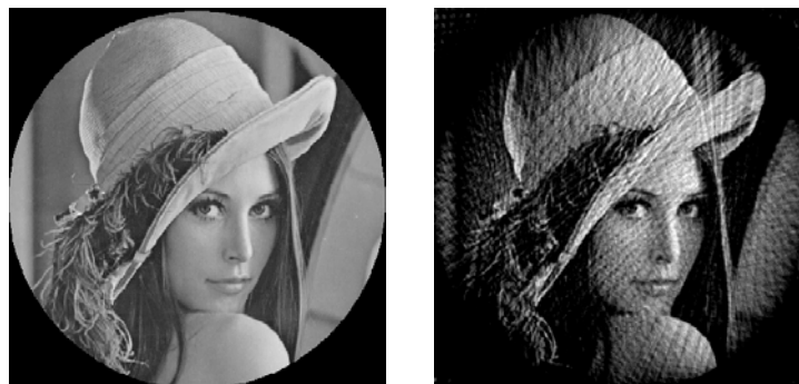
Figure 13: The original (left) and reconstruction (right) of “Lena”. The original is 440 \times 440 pixels, the aperture used has a 220 pixel radius, and 60 independent knife-edge angles are used.
